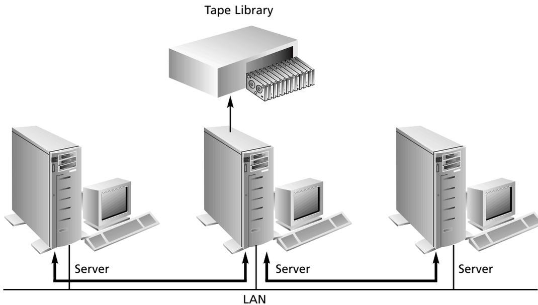
Unfortunately this approach suffers from poor performance and consumes significant network bandwidth, leading to longer backup times and reduced availability of mission critical applications while backups occur. Modern tape drive performance far exceeds the limits of modern network performance, resulting in a bottleneck caused by the network.
