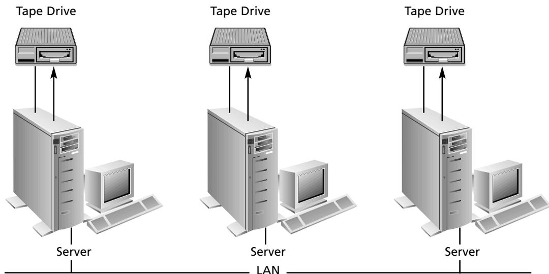
Unfortunately this approach requires extensive manpower and is difficult to automate, leading to high potential for human error. Every server must be touched on a regular (often daily) basis to ensure that media is available and the system is operating properly. In addition, this approach requires a significant investment in hardware for each server.
